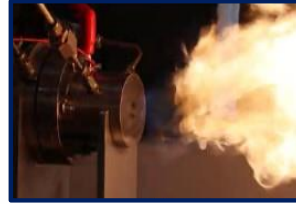
Hot Fire test of Rocket Motor in Expanse Rocket Lab
